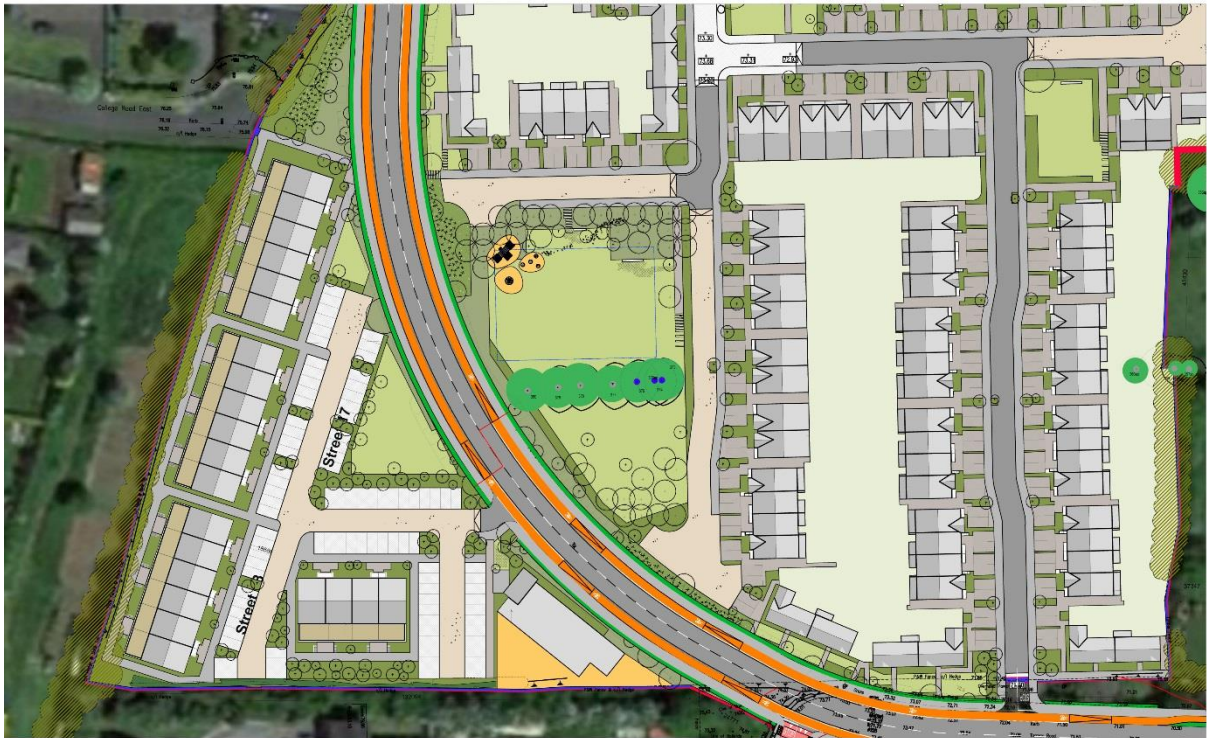
Fig 3.6- Iteration 1, above and current version, Fig 3.7 below. Three storey apartment block introduced to the eastern side of the Link Road, which is faceted to follow its curvature. The open space (No. 2) has been rotated 90 degrees, which facilitates preservation of more of the existing tree and hedgerow line running east-west. More open space is provide for north of the tree line (Open Space 6). Parking serving the apartment block is located behind the building line. The duplex blocks on the western side have been aligned with the Link Road again with parking and open space to the rear.
