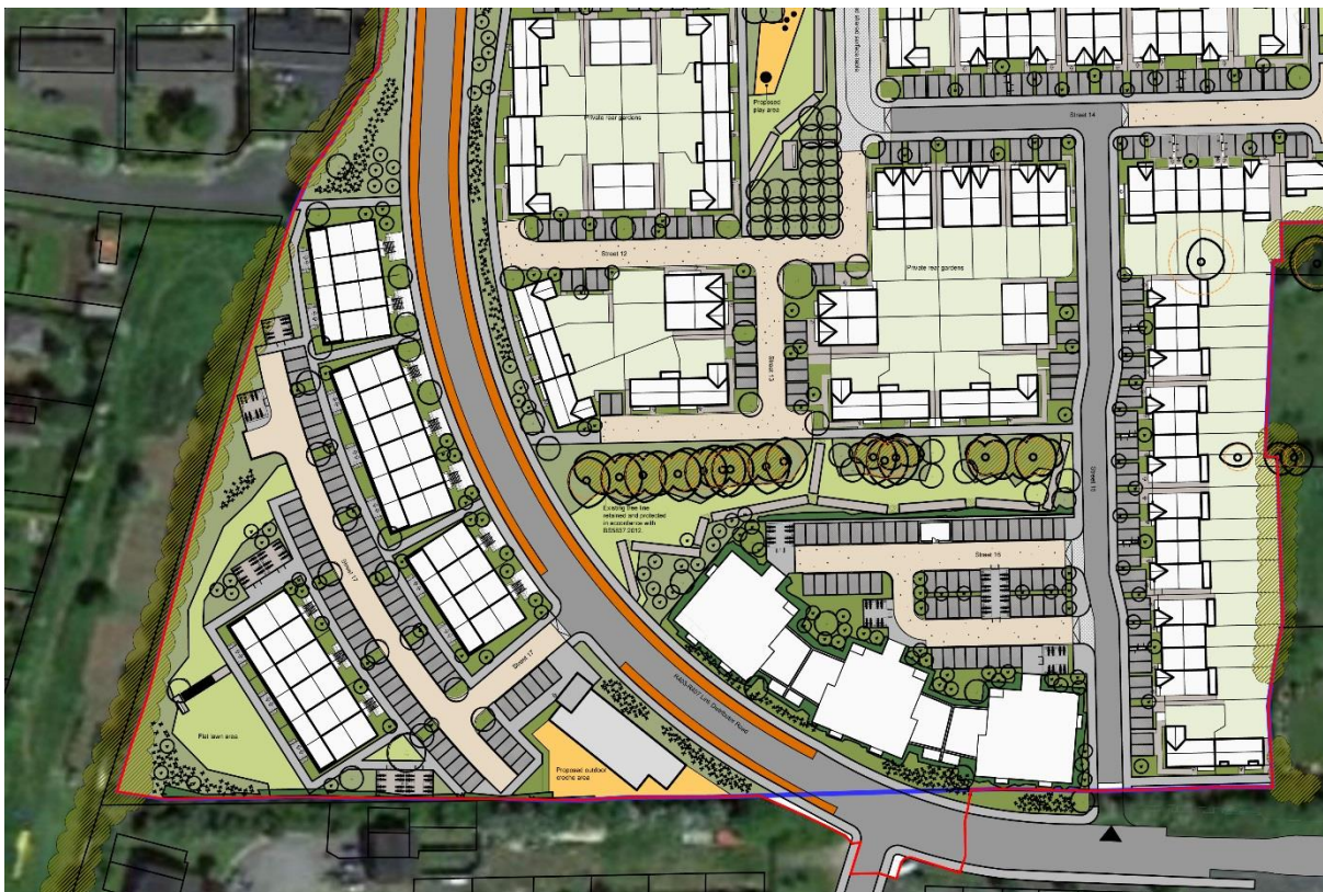
Fig 3.6- Iteration 1, above and current version, Fig 3.7 below. Three storey apartment block introduced to the eastern side of the Link Road, which is faceted to follow its curvature. The open space (No. 2) has been rotated 90 degrees, which facilitates preservation of more of the existing tree and hedgerow line running east-west. More open space is provide for north of the tree line (Open Space 6). Parking serving the apartment block is located behind the building line. The duplex blocks on the western side have been aligned with the Link Road again with parking and open space to the rear.
