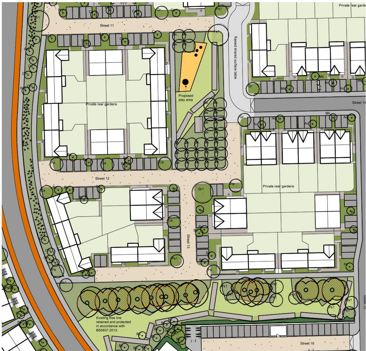
Fig 2.21 Above, Open Spaces 1 and 4 above at the heart of the development- Many of the pedestrian routes converge on these. Fig 2.22 Below, Open Space 2 focussed on the existing hedgerow line, connected both visually and physically to Open Space 6 to the north, which provides for a play area and is bounded and fully supervised by housing.
