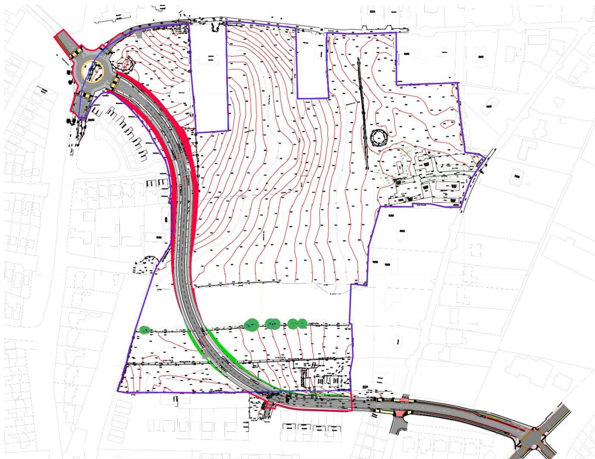
Figure 1.6 (above) showing the cut and fill and site configuration by the link road on the existing topography of the lands. Figure 1.7 (rotated view overleaf) shows an aerial view of the site identifying key constraints and opportunities presented by the site, both existing and proposed.
